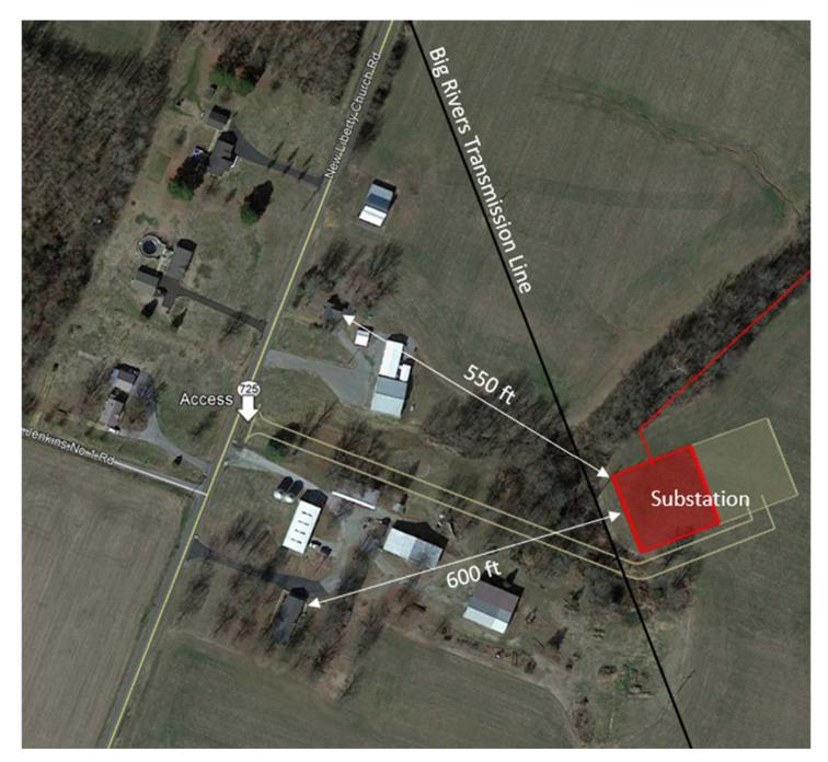
Power lines will run from the southern section of the solar farm to a new substation that will connect the solar farm to the Big Rivers transmission line. The setback between the new substation and the nearest house is in excess of 500 feet. The natural vegetative buffer at the substation location will be retained.
